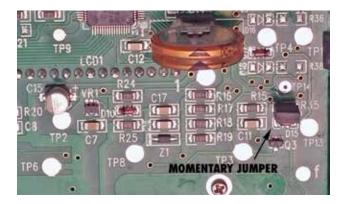
1. Upon removing the jumper and pressing the **RESET** key, the unit will be configured as a 1 channel momentary ON and OFF. ONLY CH1 will need to be programmed. CH2 can still be viewed and programmed but will not take effect.
