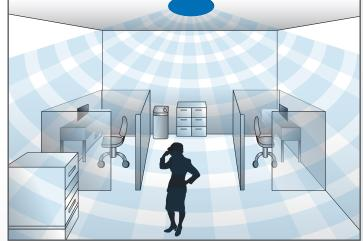
**Dual (PIR/Ultrasonic) technology** combines PIR with Ultrasonic technology. Ultrasonic utilizes wave analysis and Doppler sound waves to detect differences in energy from different phenomenon. The combination of the two technologies enhances responsiveness for maximum system reliability.
