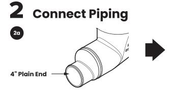
The SV10 sampling port comes from the factory ready to connect to 4" drain lines.
