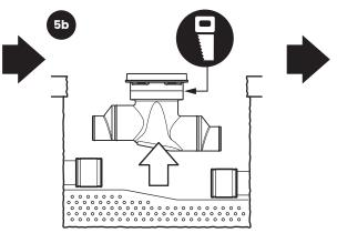
Disconnect the SV10 and remove it from the burial pit. Cut the SV10 at the Riser Cut Line, freeing the cover adapter from the sampling port body.
