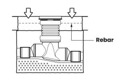
Backfill evenly around tank using crushed aggregate (approximately 3/4" size rock or sand with no fines) or flowable fill. **Do not compact backfill around unit.**
