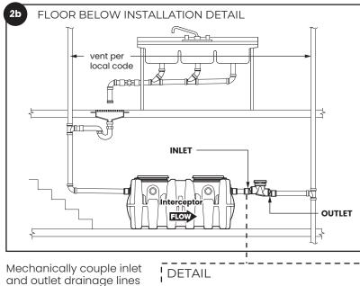
to unit. **IMPORTANT!** Make sure the sampling port is correctly aligned. The SV10 outlet is 2" lower than the inlet to facilitate sample retrieval and comply with local codes. **DO NOT install backwards as doing so will result in improper drainage slope.**
