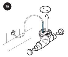
For base unit testing, cap both connection points with 4" flexible PVC caps. Remove cover and fill with water to just above the highest connection.
