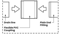
**Do not solvent weld.** Vent per local code.
