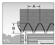
2. Add the total gutter length and the total downspout length to the figure calculated in step 1 to get the total length of cable required.
