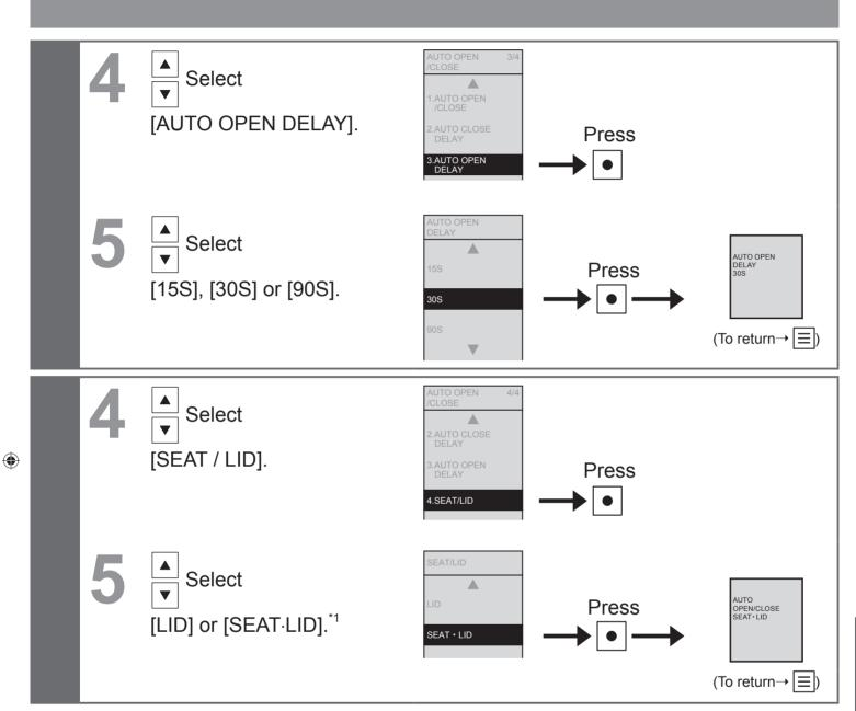
\*1 When the "Seat·lid" are set to open automatically, pre-mist is not sprayed.
