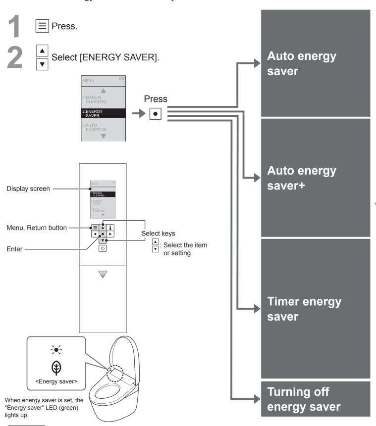
• During setting, the display goes out when no button is pressed within about 60 seconds. If you fail to complete the setting, redo from the step 1.
