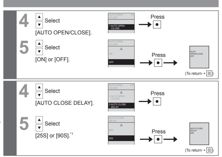
\*1 When set to "25 seconds", the lid/seat does not open automatically for about 15 seconds after closing automatically.
