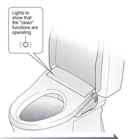
The self-cleaning functions operate automatically. (See pages 22 and 23 for details.)
