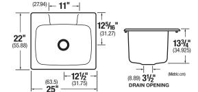
**General:** Furnish and install as shown on plans, a Countertop Sink Model 10C as manufactured by E. L. Mustee & Sons, Inc. Shall be molded fiberglass, using matched metal molds under extreme heat and pressure. One-piece molded construction with self-rimming edge. Complete drain assembly. Overall size: 22"x 25" x 13<sup>3</sup>/<sub>4</sub>". Shall meet ANSI Specification Z 124.6. Color: (White, Biscuit).
