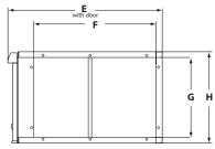
Inlet Side Return Duct Connection
