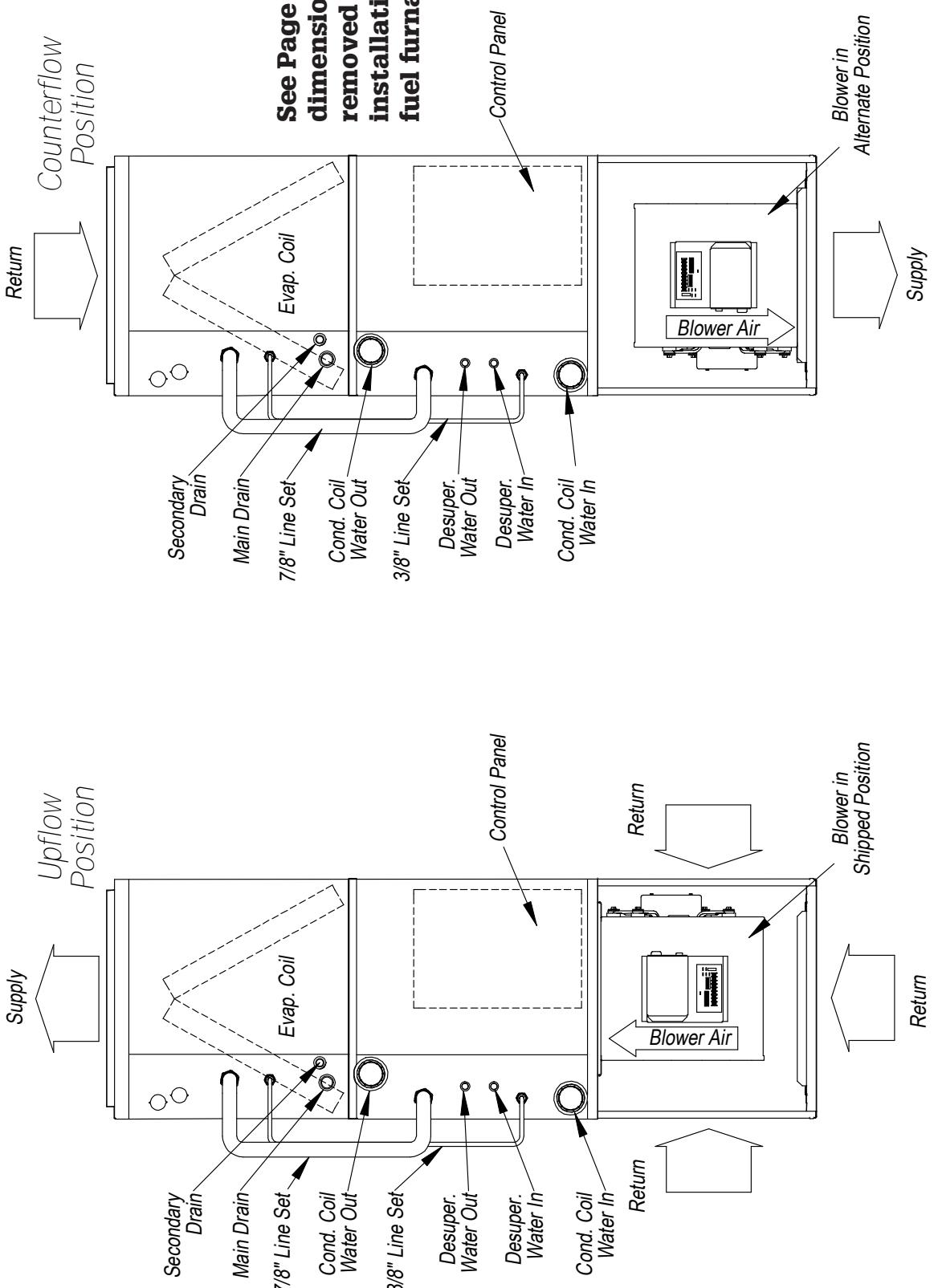
**Air Filter Required on Return Air Side for All Installations**
