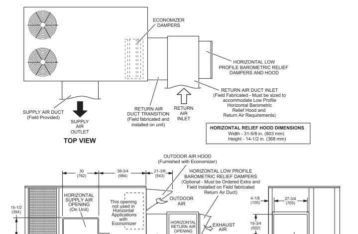
NOTE - Return Air Duct and Transition must be supported.
