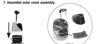
Note. Verify that rubber insert is installed
