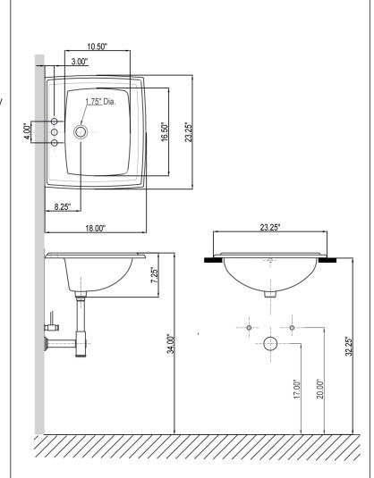
IMPORTANT: These dimensions are nominal and vary within the range of tolerances established by ASME standard A112.19.2
