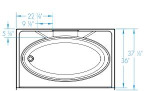
FEATURES lbs Dimensional Tolerance ± %". Dimensions needed for site preparation should be measured from the unit. Aquatic assumes no responsibility for preparatory work.
