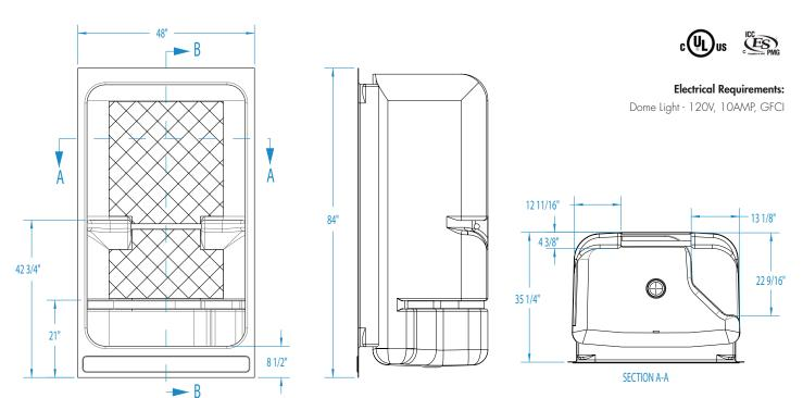
FEATURES Ibs Dimensional Tolerance ± 3/8". Dimensions needed for site preparation should be measured from the unit. Aquatic assumes no responsibility for preparatory work.
