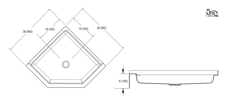
FEATURES Ibs Dimensional Tolerance ± 36". Dimensions needed for site preparation should be measured from the unit. Aquatic assumes no responsibility for preparatory work.
