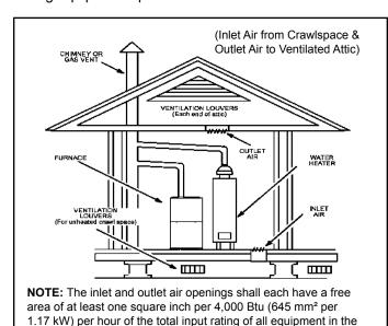
Figure 4. Equipment in Confined Space - All Air from Outside
