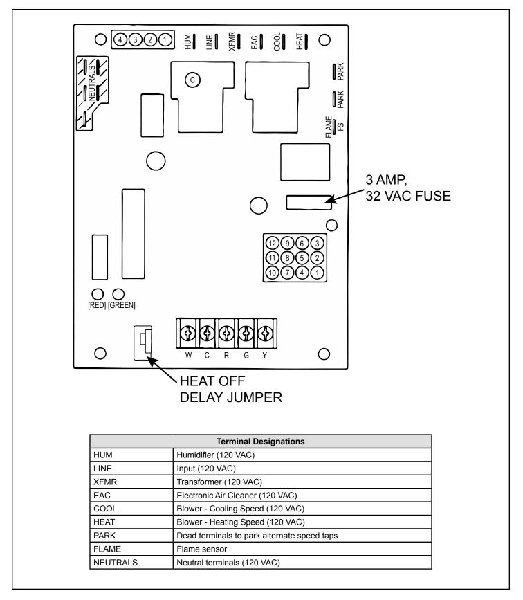
Figure 26. Integrated Control (Automatic Hot Surface Ignition System)
