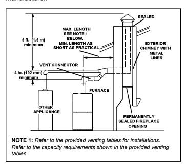
Figure 17. Common Venting Using Metal Lined Masonry Chimney
