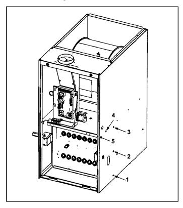
Figure 32. Remove 5 Screws if Necessary
