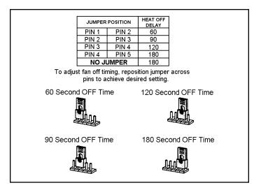
Figure 29. Heat Fan Off Time in Seconds
