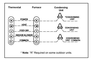
Figure 23. Condensing Unit Thermostat Designations
