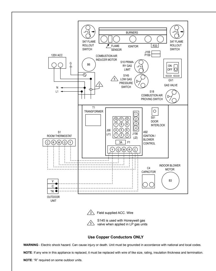
Figure 25. Typical Field Wiring Diagram
