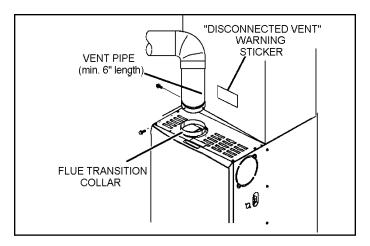
Figure 16. Vent Connection
