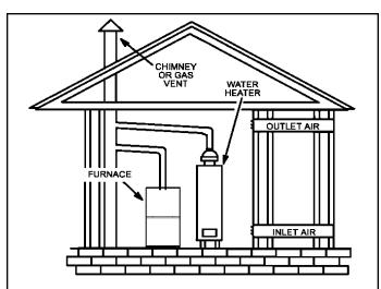
**NOTE:** Each air duct opening shall have a free area of at least one square inch per 2,000 Btu (645 mm² per .59 kW) per hour of the total input rating of all equipment in the enclosure. If the equipment room is located against an outside wall and the air openings communicate directly with the outdoors, each opening shall have a free area of at least 1 square inch per 4,000 Btu (645 mm² per 1.17 kW) per hour of the total input rating of all other equipment in the enclosure.
