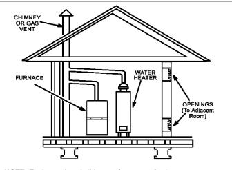
**NOTE:** Each opening shall have a free area of at least one square inch per 1,000 Btu (645 mm² per .29 kW) per hour of the total input rating of all equipment in the enclosure, but not less than 100 square inches (64546 mm²).
