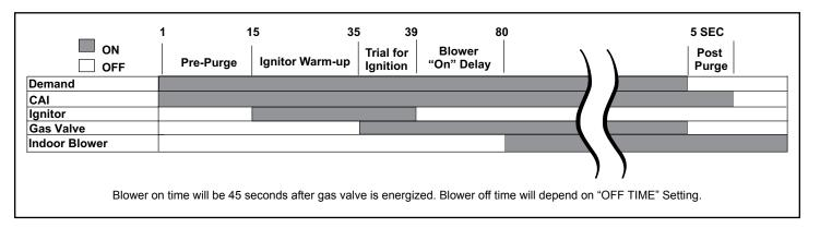
Figure 28. Integrated Ignition Control
