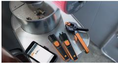
With the Heating set, you can determine gas flow and static pressure, measure temperature of radiators, and much more
