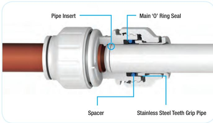
John Guest Twist and Lock® Fittings have a collet with stainless steel teeth that grip the pipe when fully inserted, and an O-ring to provide a permanent leak-proof seal. The additional benefit of the Twist and Lock fitting is that a twist of the screw-cap gives greater compression on the O-ring seal and locks the pipe in place for greater security.
