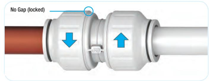
Twist the screw-cap until it touches the body flange. This locks the pipe into position and increases the o-ring seal around the pipe.
