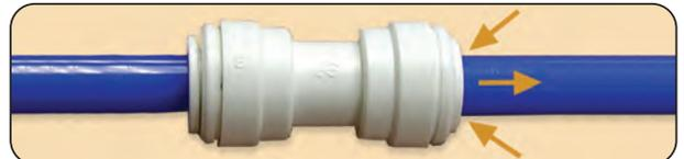
To disconnect, ensure that the system is depressurized, push the collet square against the fitting. With the collet held in this position the tube can be removed.
