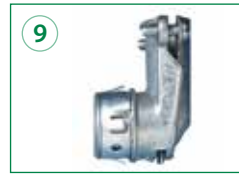
9 Size: 3/8": P/N E00-015-000 1/2": P/N E00-005-001 Type: Snap-in, 90° Material: Die Cast Insulated: No
