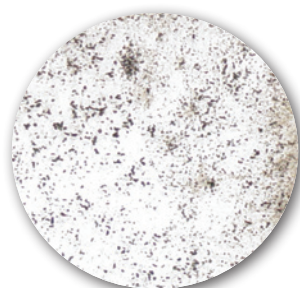
Standard plastic pan with visible mold
