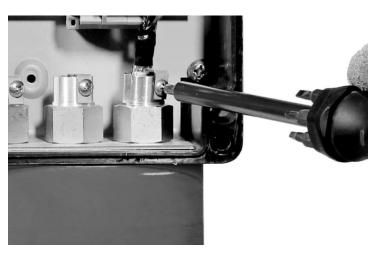
PGW/MT only: Place the supplied tube over one bus wire prior to sliding the core sealer over the bus wires. This will provide added protection from a short between the two bus wires (see inset).
