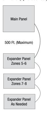
Daisy Chain Zones Located Remote to Main Panel - Remote Panels Wired in Star Configuration
