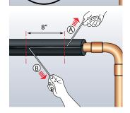
5. Remove the white release paper strip in 8" increments, by drawing it away from the insulation.
