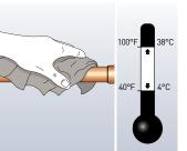
1. Clean all dust, dirt, oil and water from pipework using denatured alcohol where necessary. Install Armaflex when ambient temperature is between 40°F (4°C) and 100°F (38°C).
