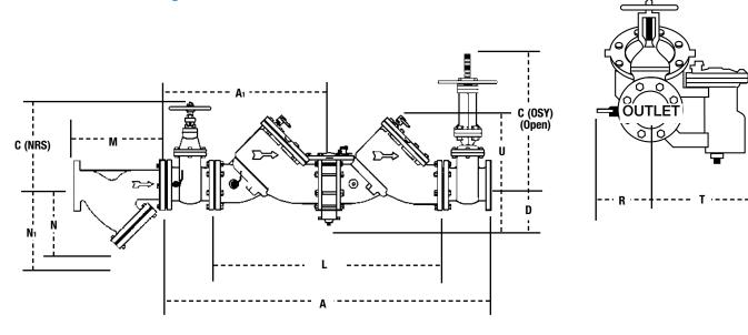
Note: Relief valve section is reversible, therefore, can be on either side and is furnished standardly as shown.
