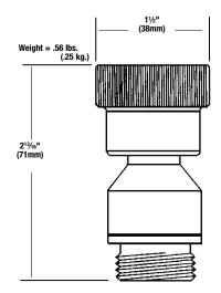
In-line field testable - no special gauges requiredManually drainable for freeze protection
