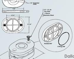
Cleanout Slips over SDR-35 Pipe
