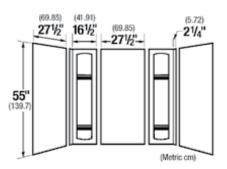
**General:** Furnish and install as shown on plans, DURAWALL\* Bathtub Wall Model 950, as manufactured by E.L. Mustee & Sons, Inc. The white thermoplastic wall system shall be 5-piece construction with four formed shelves. One-piece, seamless comer panels with overlapping edges. Uniform color throughout entire thickness of each panel. Color: White.
