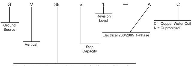
38 = Nominal heating capacity in thousands @ 50° water - Full Load Nominal cooling capacity in thousands @ 77° brine - Full Load
