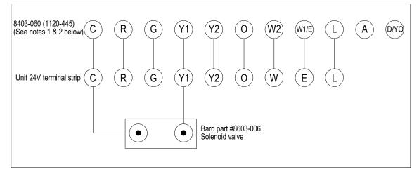
1. Will need to be programmed for multi-stage heat pump 2. Will need to be configured to energize reversing valve for cooling mode
