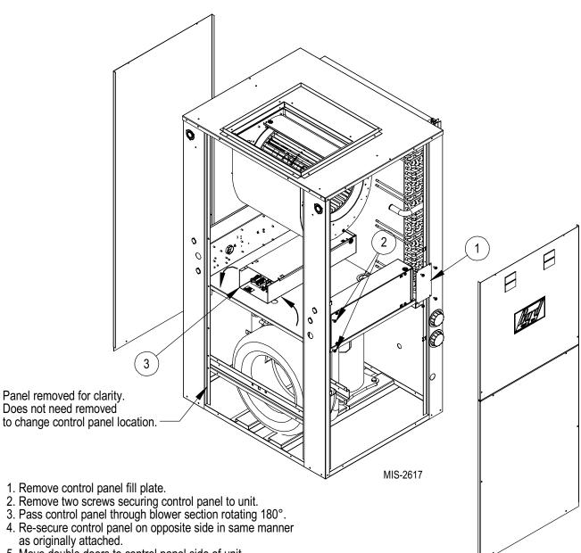
5. Move double doors to control panel side of unit.
