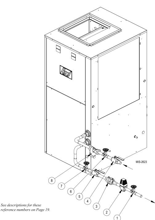
FIGURE 10 WATER CONNECTION COMPONENTS
