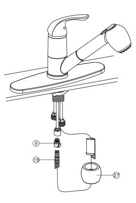
3.Fix the weight ⑦ to the pull-out hose(), and connect the pull-out hose () to quick connect assembly(). CAUTION: MAKE SURE THE HOSE IS PROPERLY ENGAGED AND SECURED IN THE QUICK CONNECT ASEEMBLY.
