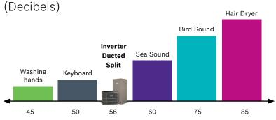
The lowest average sound rating is 56dB for the Inverter Ducted Split 3 and 4 Ton unit. Based on a weighted overall (dB), according to ARI-260:2001(100hz-10kHz). Actual sound rating may vary depending on system setting, equipment maintenance, and other factors that may affect the sound rating.
