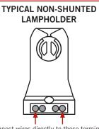
Connect wires directly to these terminals
