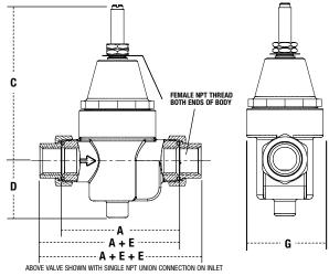
VALVES MAY BE ORDERED WITH 0,1,0R 2 UNION CONNECTIONS USING ANY COMBINATION OF NPT, SOLDER, PEX OR CPVC CONNECTIONS REQUIRED
