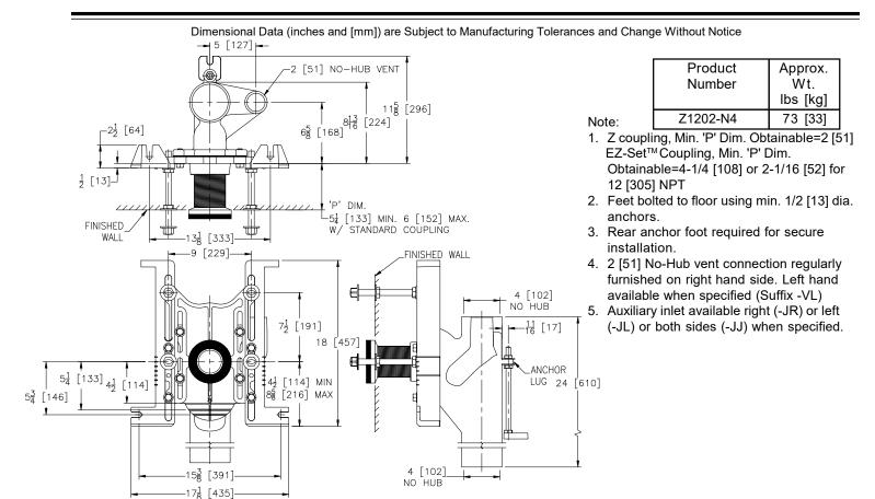
SIPHON JET NO-HUB WATER CLOSET CARRIER SYSTEM
