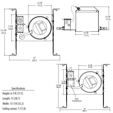
All dimensions are inches (centimeters) unless otherwise specified. **option 277V step down transformer**
