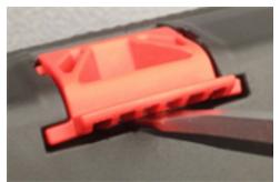
To remove a damaged lock system, flip tote upside down and approach tote from the bottom of base. Insert a large flat blade screwdriver in middle of locking carriage as shown. Lightly pry carriage upward out of base opening. Remove and discard old locking carriage and spring.
