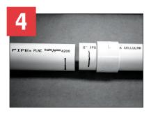
coupling has raised quarter mark lines on the outside diameter of the coupling.)
