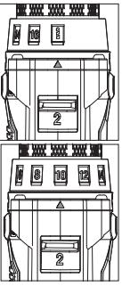
2. To use the driving mode rotate the torque selector collar until the desired clutch setting appears in line with the arrow.
