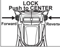
1. For forward (clockwise) rotation, push in the control switch from the right side of the tool. Check the direction of rotation before use.
