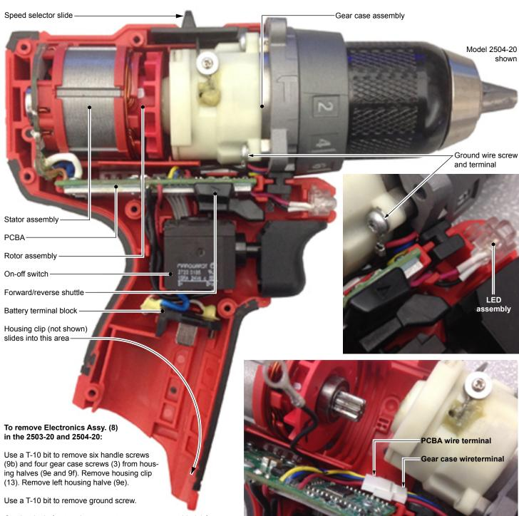
Gently wiggle front end to separate gear case assembly (4) from pinion of rotor assembly (6). Carefully disconnect male/female wire terminals to separate gear case assembly from PCBA.
