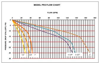
NOTE: Although this chart shows curves at a 50 psi set differential, curves for other settings are similar. The curve shifts sightly to the left for a smaller differential and to the right for a greater differential. The adjustment is as follows: for a 25 psi set differential subtract 15% from the flow rate shown. For a 75 psi set differential add 15 % to the flow rate shown.
