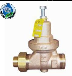
Apollo PR Series pressure reducing valves provide automatic control of excessive water pressure and problem supply fluctuations. These models are designed to reduce pressures of up to 300 PSI to a more manageable range.
