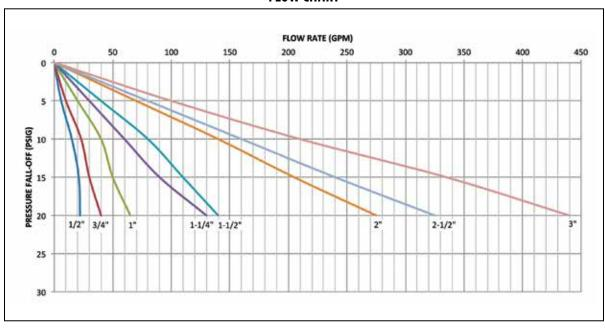
NOTE: Flow curves are based on static conditions of: Inlet pressure = 100 psig: Outlet pressure = 50 psig. All curves are for female NPT versions only. Fall Off is the difference between the PRV's set pressure and the flowing pressure at any given demand.
