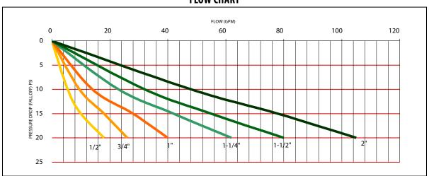
NOTE: Flow curves are based on static conditions of: Inlet pressure = 100 psig: Outlet pressure = 50 psig. All curves are for female NPT versions only. Fall Off is the difference between the PRV's set pressure and the flowing pressure at any given demand.
