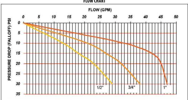
Fall Off is the difference between the PRV's set pressure and the flowing pressure at any given demand.
