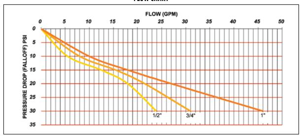
NOTE: Flow curves are based on static conditions of: Inlet pressure = 100 psig: Outlet pressure = 50 psig. All curves are for female NPT versions only. Fall Off is the difference between the PRV's set pressure and the flowing pressure at any given demand.
