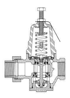
Fall-off is the reduced pressure change that results when a valve opens: the difference between the static (closed) pressure and residual (flowing) pressure downstream of the regulating valve. Inherent in the direct-acting design, fall-off is an important factor when choosing a valve size and type.
