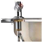
Step 1: Insert flex line inlets and tighten by hand. Apply plumber's putty to underside of body and insert into mounting hole. With wrench, tighten the locking nut.
