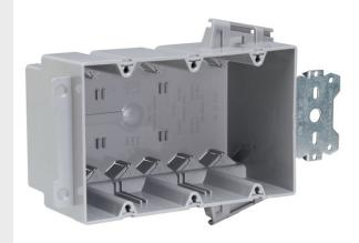
Triple Gang, Wood and Steel Stud Bracket Box with Quick/Click. 3/8" offset for wood and steel stud mounting. Six Auto/Clamps on each end. For use with 3/8" to 5/8" wallboard.
