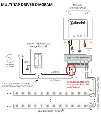
† Install a compatible magnetic low voltage dimmer switch. See dimmer switch manufacturer installation guide for complete wiring instructions.
