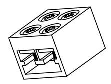
Ribbon insertion end, with positive contact set screws
