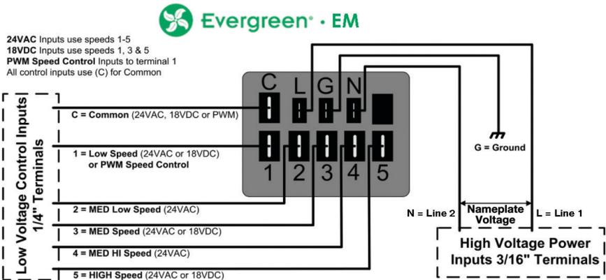
Detailed wiring for the High Voltage Power Connections and each unique Low Voltage Signal Connections are covered in the following sections.
