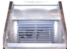
The blower wheel hub locking bolt should be secured to the flat portion of the motor shaft after the wheel has been centered in the blower housing.
