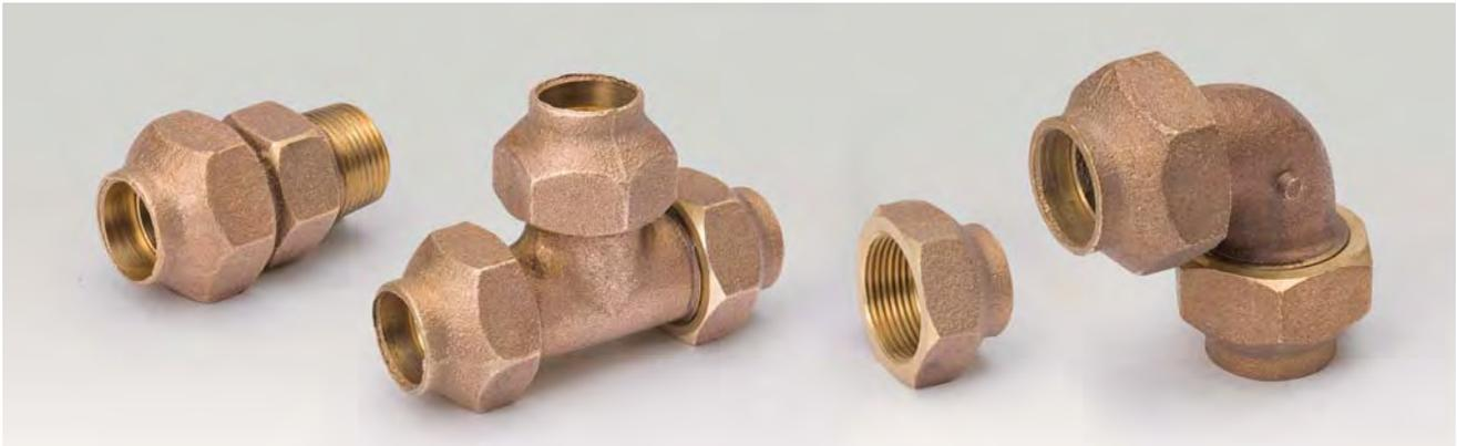
Streamline® Copper Flare Fittings are for use with above-ground flexible copper tube in common potable water supply systems. These fittings make for easy and flame-free installations and require common tools for assembly. Available in five diameters from 1/2" to 2", these flare fittings come in an assortment of styles to meet common job needs.
