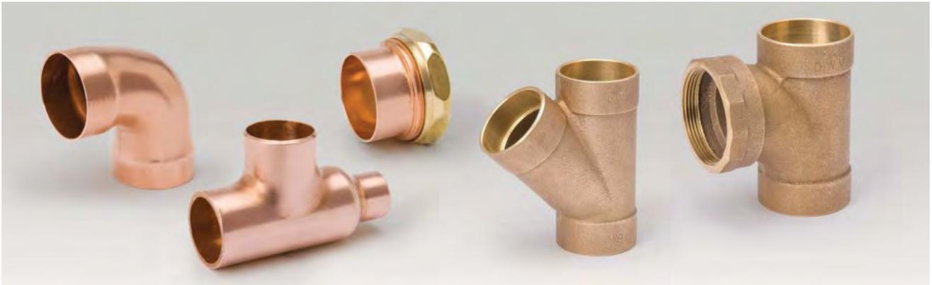
Streamline® Copper Solder-Joint Fittings for DWV plumbing applications are available in both wrot copper and cast bronze materials. Designed for use in non-pressurized sanitary systems, these fittings commonly feature shorter solder cup designs and more sweeping turns. They are available in a wide range of diameters, styles and connections to meet most all sanitary system applications.
