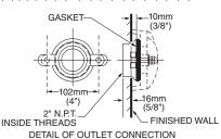
FLUSH VALVE NOT INCLUDED WITH FIXTURE AND MUST BE ORDERED SEPARATELY. PROVIDE SUITABLE REINFORCEMENT FOR ALL WALL SUPPORTS.
