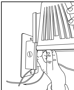
Slide fixture housing onto mounting box
