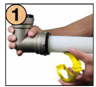
Shark Shifter De-Mount Tool to pipe just above the connection then slide down to engage lugs on the head of the fitting.
