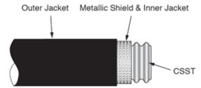
Note: Care is needed to avoid cutting through the aluminum shield during this jacket layers stripping step. Cutting through the aluminum shield below the point of the outer jacket cut/strip location will reduce the effectiveness of the fitting-to-shield electrical continuity, and FlashShield's electrical performance.
