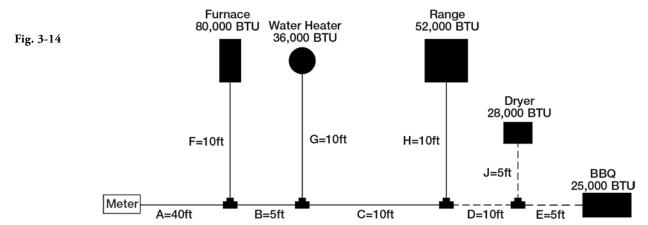
Note: Rigid pipe sized using a 0.5"WC pressure drop table, as no 2.0"WC pressure drop table for Rigid pipe is available.
