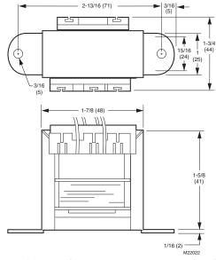
AT120 Transformer dimensions in in. (mm).
