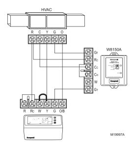
Fig. 4. Wiring heat pump without emergency heat.
