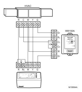
Fig. 1. Single transformer, conventional system.
