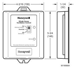
W8150A Ventilation Control dimensions in in. (mm).
