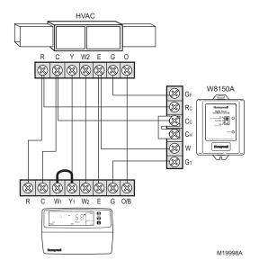
Fig. 5. Wiring heat pump with emergency heat.
