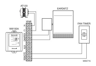
Fig. 7. Using a remote switch or timer.
