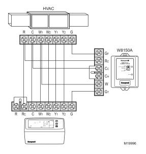
Fig. 3. Multi-stage conventional system.
