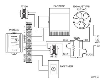
Fig. 9. Wiring an exhaust fan.
