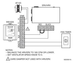
Fig. 8. Wiring to an HRV/ERV.
