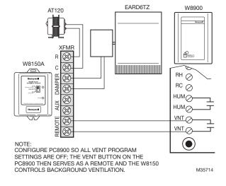
Fig. 6. Wiring with a PC8900.
