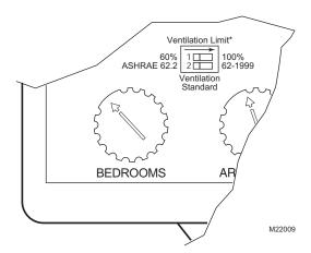
Setting ventilation limit and ventilation standard.
