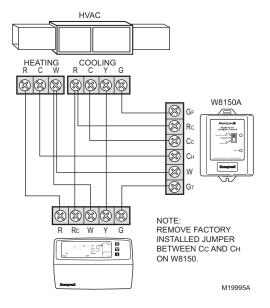
Fig. 2. Dual transformer, conventional system.
