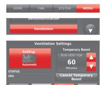
NOTE: If set up for humidification in heat mode. the ventilator will turn on to remove excess humidity if 10% or more above your humidity setting.
